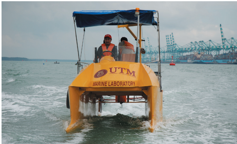
Manoeuvrability testing of Semi-SWATH prototype
